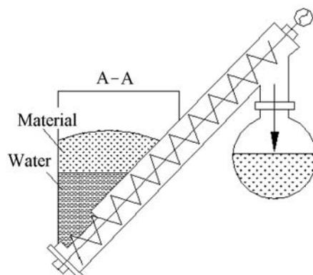
Fig. 2. Screw-conveyor loading of the reactor with a water-seal bin.
