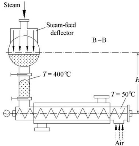
Fig. 3. Screw-conveyer unloading of the reactor with sluice gates and cooling.
